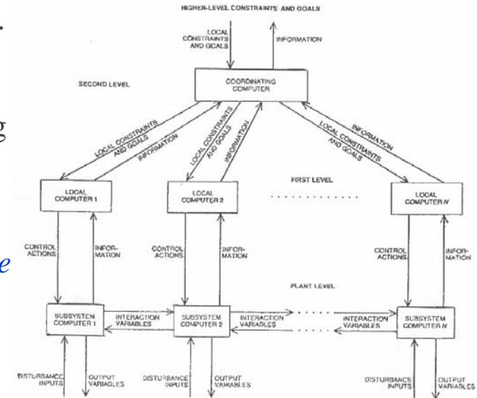
Fig. 6 The well-known hierarchical, computer control based, implementation of integrated control and supervision [214] for complex dynamic networks and systems in terms of dynamic sub-networks of nonlinear dynamic nodes, which in compliance with Siljak's concept of dynamic graphs (2008).
