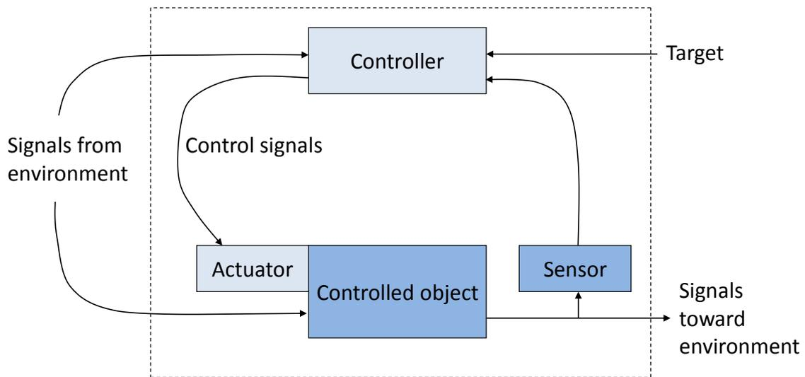
**Figure 1.** Diagram of a self-controlled system
