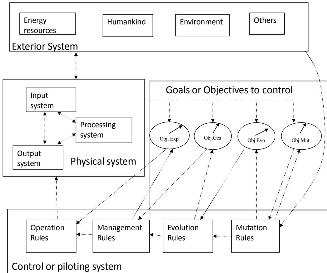
**Figure 4.** Diagram of the ultra-stable system of Ashby applicable to the case of an intelligent system
